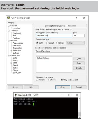
Figure 5-1: IXT-900-2X1UP SSH Login Screen
